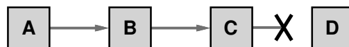
Figure 2: An example of DSR Route Maintenance. When forwarding a packet from node A to node D, node C detects that the next link along the source route (the link from C to D) is broken and returns a ROUTE ERROR to node A, the original sender of the packet.
